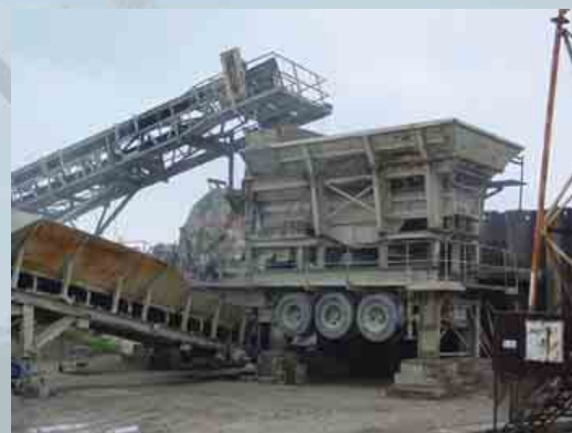
Figure 3 Station crushing and separation system
